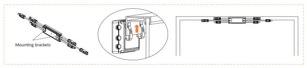
NOTE: Do not place the RSD-D (including DC connectors) where exposed to the sun, rain or snow, even gap between modules. Any surface of the RSD other than the mounting bracket must be at least 15mm away from surrounding objects. In particular, it is forbidden to have DC cables run close to or cover the RSD casing.
